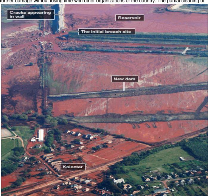
the road leading to the reservoir was done and backfilling of reservoir wall undertaken to prevent further leakage.
